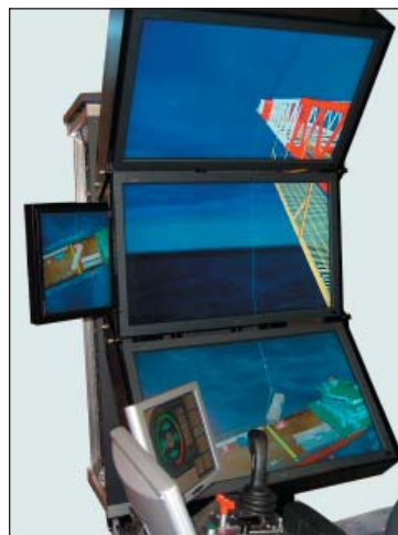
The DrillsIM-600 in "vertical" mode for offshore pedestal crane operator training
